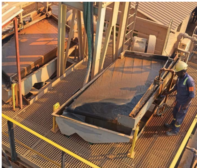
Simple gravity separation to produce rare earth concentrate at Rainbow Rare Earths' Gakara Project in Burundi, East Africa.
